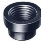
Dramm threaded gasket with 3/8" Witworth thread. Use at pressures up to 50 psi. Drill 7/16" hole in PVC pipe or cap and install insert. Insert is then ready to accept nozzles and screwing in the nozzle will tighten or compress the insert securely in place.
